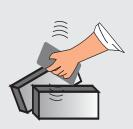
Before application clean the surface of blocks using suitable tools like blush so that any foreign material is not held on the blocks.
