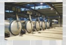
It is further strengthened by high pressure steam curing in Autoclaves.
